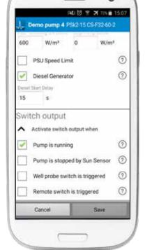
With the enhanced software features most of the irrigation process is handled automatically according to the pump configuration.
